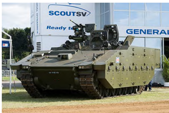
The FRES Scout SV is a new family of tracked specialized vehicle that is replacing the Saxon, FV432 and CVR(T)
